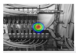
FIND LEAKS FASTER Detect compressed air leaks up to 10 times faster with sound imaging vs. traditional methods
